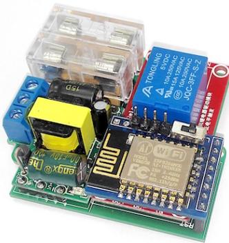
Fig. 6: The finished control unit hardware.
